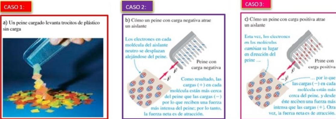
Figure 5.6: Electrization by induction.
