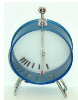
Figure 2.1: Electroscopio
